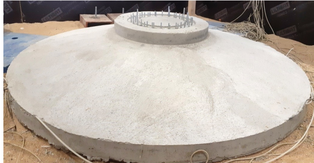
1/10 scale model of a foundation. Tests carried out at INSA Lyon.
